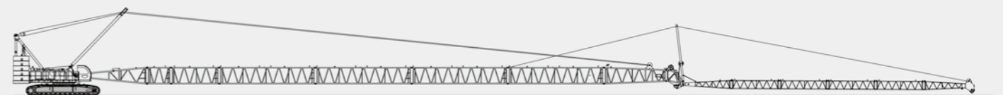
塔式副臂安装示意图 Tower jib installation illustration
