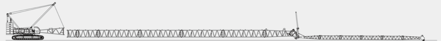
固定副臂安装示意图 Fixed jib installation illustration
