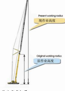
作业高度拓展 The lifting height is increased
