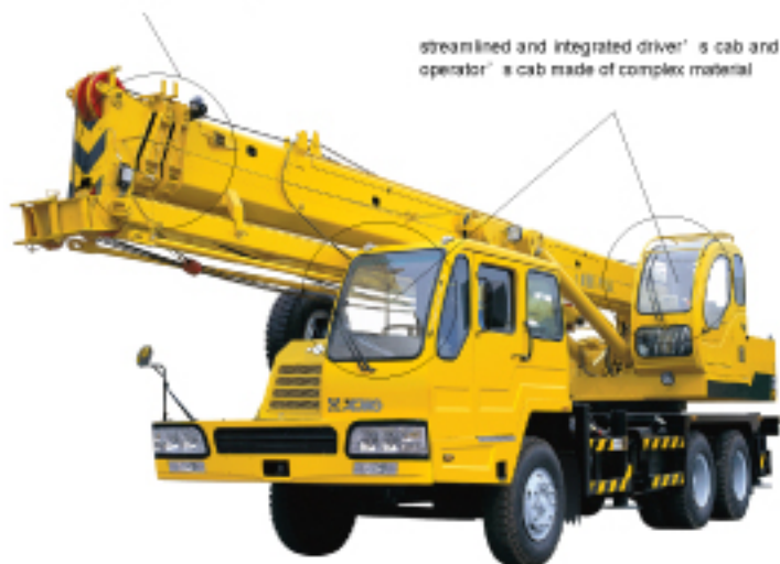
3-section hexagonal telescopic boom
