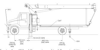
Requires front SFO stabilizer to give machine full capacity 360° around the truck. Truck must meet the minimum requirements above. Front stabilizer gives the machine a solid base, helping the operator control loads precisely.
