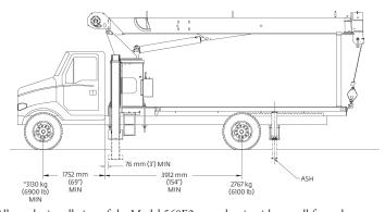
Allows the installation of the Model 560E2 on a chassis with a small frame by using the standard sub-base for 18 ft bed. In most cases, the chassis will not require reinforcing, and the amount of counterweight required is minimized, increasing payload capacities.
