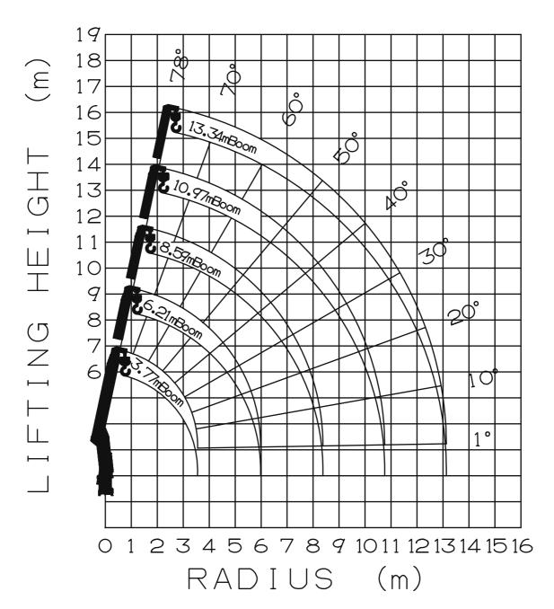
NOTE: The above lifting heights and boom angles are based on a straight (unladen) boom, and allowance should be made for boom deflection obtained under laden conditions.
