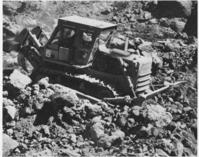
Shown with optional ROPS Modular Cab, (canopy is standard in U.S.A.), rear screen, heavy-duty radiator guard, track roller guards, fast-fill fuel system, hydraulic control, 8S Bulldozer and multishank ripper.
