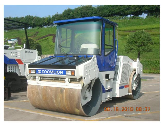
YZC13H vibratory roller is of double-drum and tandem type, suitable for asphalt concrete, gravel mixed material and harsh concrete. It is the ideal equipment for high-level road, civil road, airport, parking lot, constructional site.
