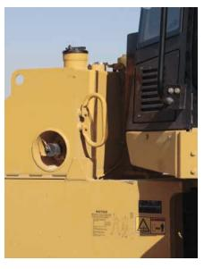
**Fuel Tank.** Is easy to reach and is positioned away from debris for protection and maximum capacity.
