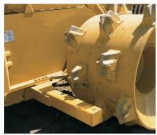
**Striker Bars.** Located in front of and behind the rear wheels and behind the front wheels provide substantial protection from trash that can be thrown or carried by the wheels.
