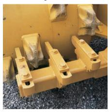
**Optional Wheel and Tip Cleaner Fingers.** Welded onto the standard striker bars, these adjustable fingers keep the wheels from plugging when working in cohesive materials such as clay or mud.
