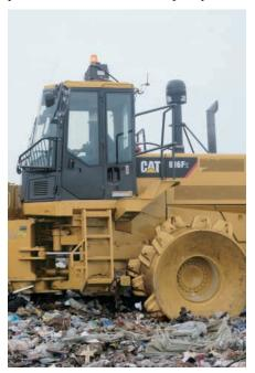
**Left Side Platform.** Rear cab access is easier with the left side platform.
