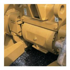
**Standard Axle Guards.** Prevent trash build-up on the axles, protect the axle seal guards and help prevent duo-cone seal failure.
