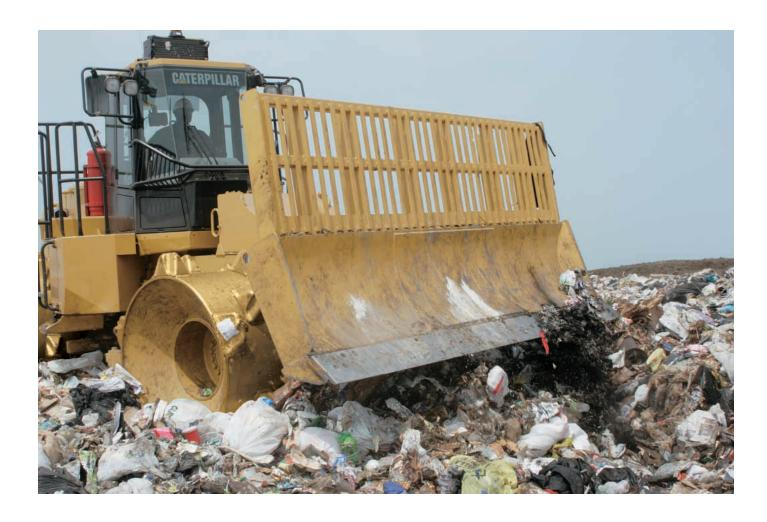
**Straight Blade.** The straight blade is a standard attachment and an ideal blade for most waste management applications.
