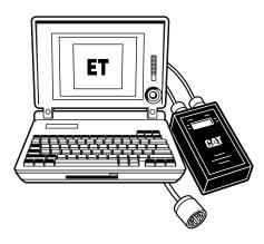
**Cat Electronic Technician (ET).** Cat ET is a software program which allows the service technician to find and identify a problem on a machine and analyze how to fix it quickly. It has the capability to access the Electronic Control Modules from a laptop computer.
