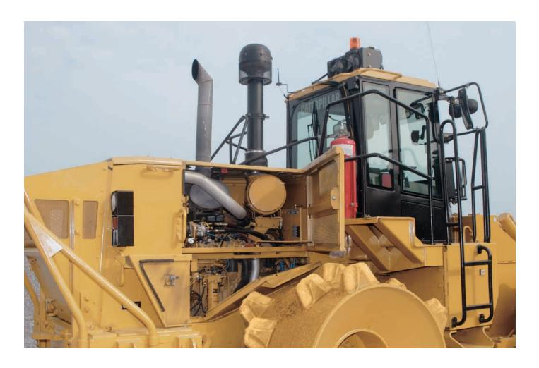
**Engine Access.** An all metal engine enclosure and hinged access doors allow for easy daily maintenance and inspection.
