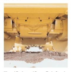
Hinged Engine and Power Train Guards. Help prevent trash build-up and shield components from demolition debris, trash, wire, rebar and harmful chemicals
