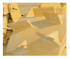
**Self Cleaning Chopper Wheels.** The self cleaning chopper wheels are designed to deliver maximum compaction and traction. Aggressive chopping action is provided by 20 blades per wheel. Heat-treated DH-2<sup>TM</sup>, ARM steel blades provide longer wear.
