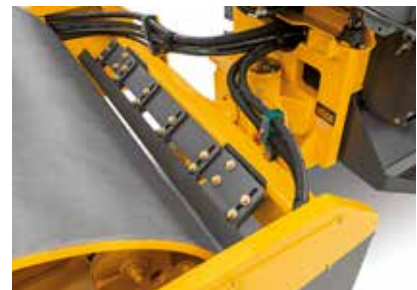
Inside drum scraper
