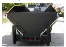
If the jobsite conditions don't permit the material feed by rear dump trucks the hopper can also be charged from the side (by conveyor, wheel loader etc.). The front hopper wall avoids spilling material in front of the paver.
