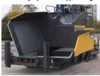
Separately controlled hopper wings facilitate feeding from the side by wheel loaders etc. when paving close to an obstruction.
