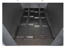
With the two independent conveyors the flow of material can be adapted to unequal requirements of each screed side (e.g. when paving along a wall).
