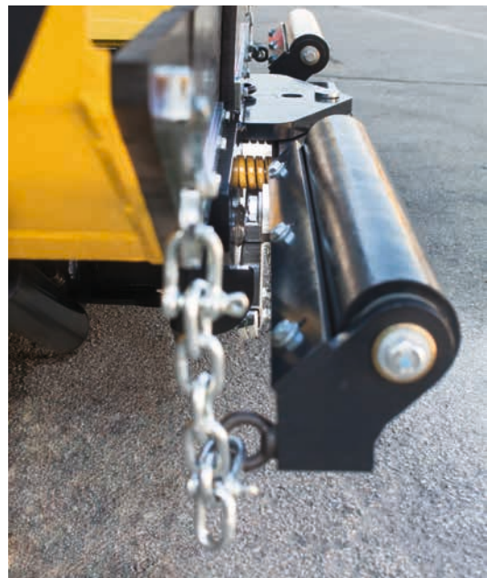
Impact-free docking – dampened bumper.
